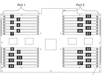
DIMM error LEDs / are built into each handle
